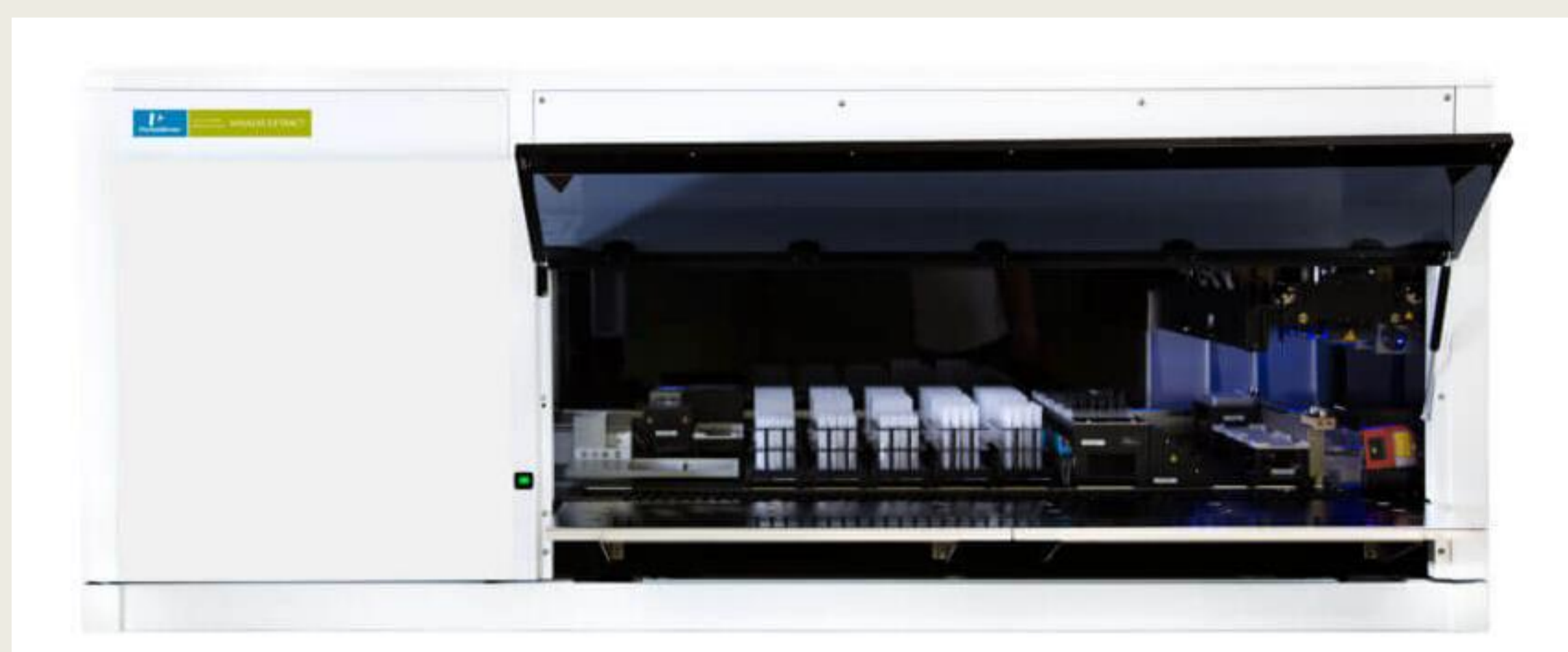
Figure 1. Vanadis Extract ® Cell-Free DNA Extraction Unit was used for automatic cffDNA extraction from plasma samples.
